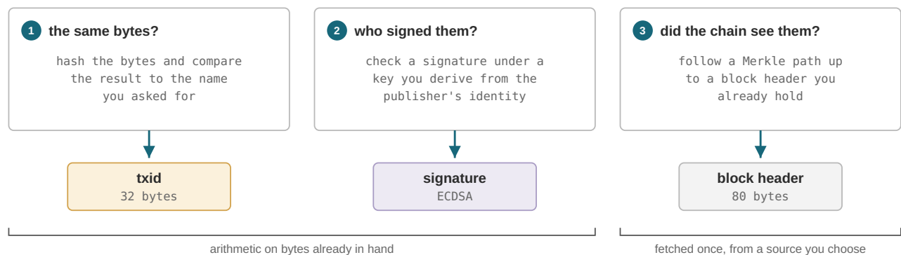
Figure 1 - the three questions. The first two are settled by arithmetic on bytes in hand; only the third needs something from outside, the block headers, and those you fetch once from a source you choose.
